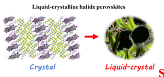
Figure 1: Schematic illustration of the solid-crystalline structure of the developed perovskites and the revealed thermally triggered liquid-crystalline phase imaged under a polarized optical microscope (POM).
