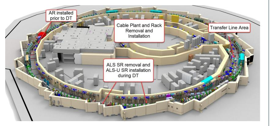
The AR is installed on the inner wall of the tunnel. Ground based bottom-up lifting and overhead crane installation methods are utilized. Preparation activities are performed before the main installations. Installation processes are guided and documented by QA procedures.
