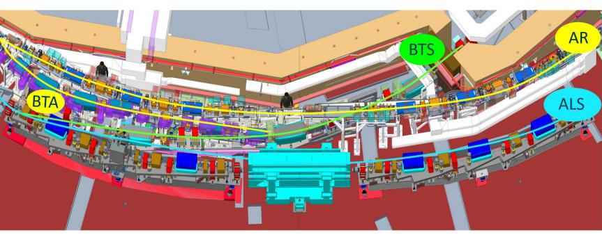
The ALS transfer line (TL) area with the Booster-to-Accumulator branching off the existing Booster-to-Storage ring TL
