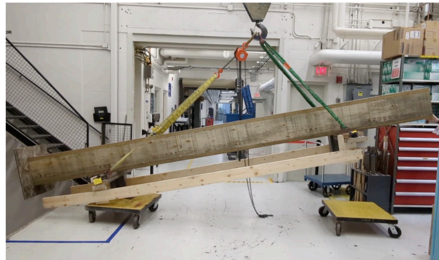
Figure 7. Test lift with wooden accelerator section mock up.
