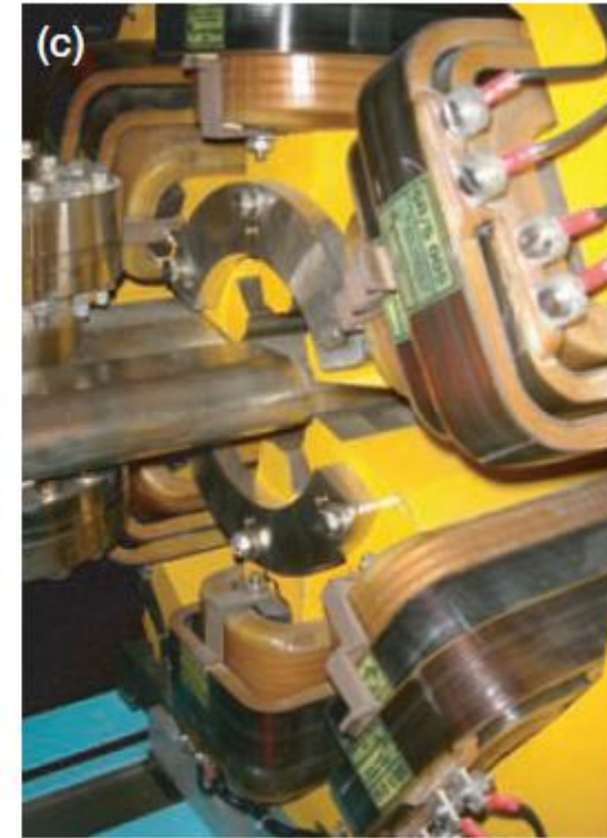
Sextupole-magnets They correct the chromatic aberration that arise from focusing by the quadrupoles
