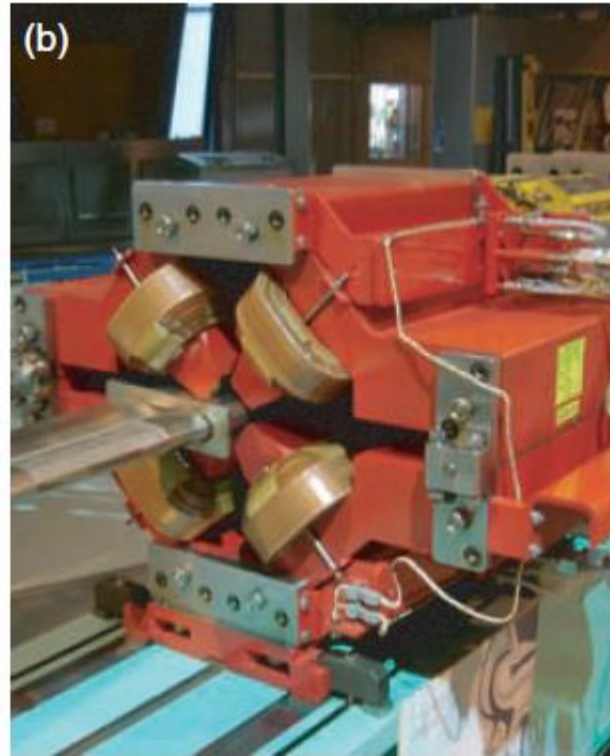
Quadrupole-magnets They are used to focus the electron beam and for Coulomb repulsion between electrons
