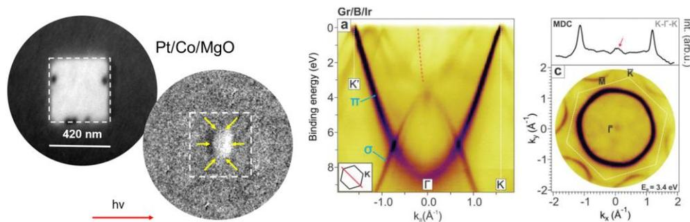
From left to right. Co  $L_3$  edge XAS-PEEM and XMCD-PEEM images of a Pt/Co/MgO nanostructure. The first image shows the lateral size of the Co square. The second image shows the magnetic fingerprint of a skyrmion, a non-trivial magnetic structure that has attracted huge scientific attention in the past years [1]; PEEM is ideally suited to perform microspot-ARPES measurements on layered materials: the example on the right hand side of the figure shows the electronic structure of Gr/B/Ir(111).
