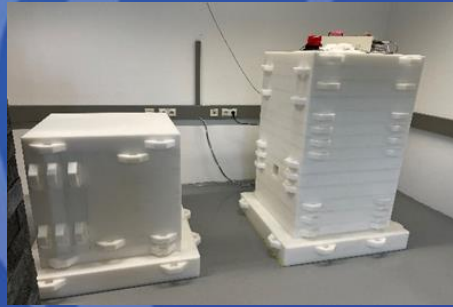
DD-type generator, with compact shielding
