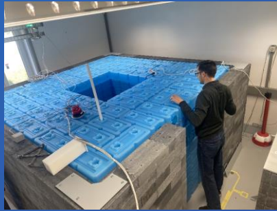
DT-type generator, with massive shielding
