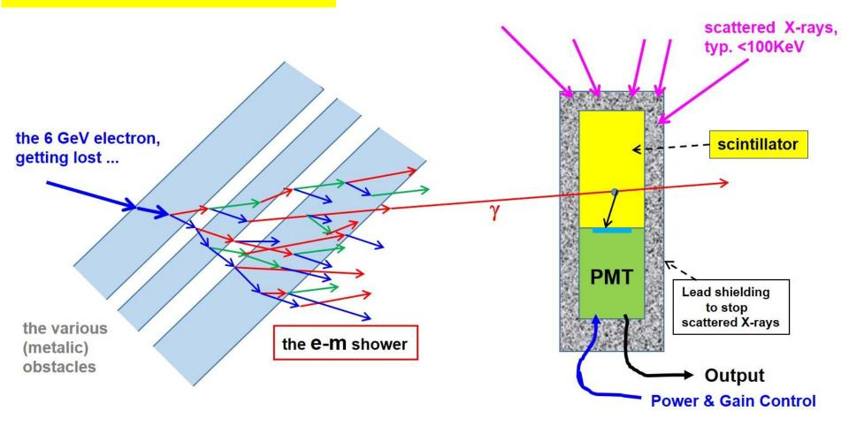
the input signal to the photo-multiplier-tube (PMT) is a pulse of about **30 picosec**, for **high amplitude** of that **short pulse** the **PMT** may **no longer be linear .....**
