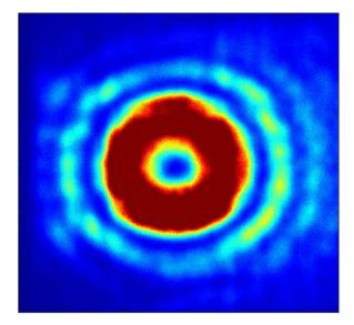
interference pattern of Visible Light produced by the fringe (slope) fields of two Dipole magnets
