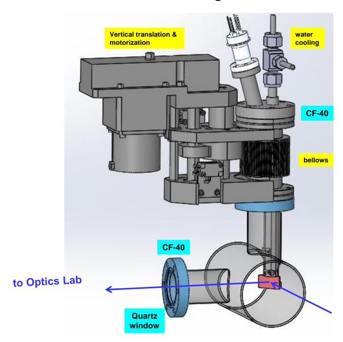
this mirror can be fully inserted into the beam-path
