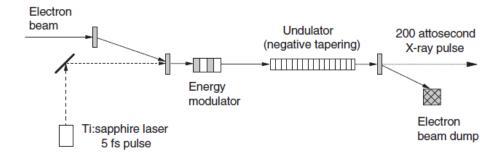
$$\frac{1}{H_{\text{w0}}} \frac{dH_{\text{w}}}{dz} = -\frac{1}{2} \frac{(1 + K_0^2)^2}{K_0^2} \frac{1}{\gamma_0^3} \frac{d\gamma}{cdt}$$
