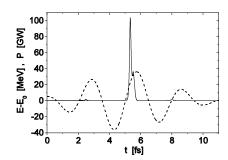
Undulator taper compensates for energy chirp within a short slice, lasing in the rest of the bunch is suppressed by uncompensated taper.
