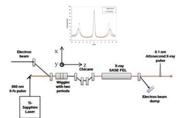
In the chicane the laser-induced energy modulations are converted into density modulations (current spikes). The spike with the highest current lases better (enhanced SASE).
