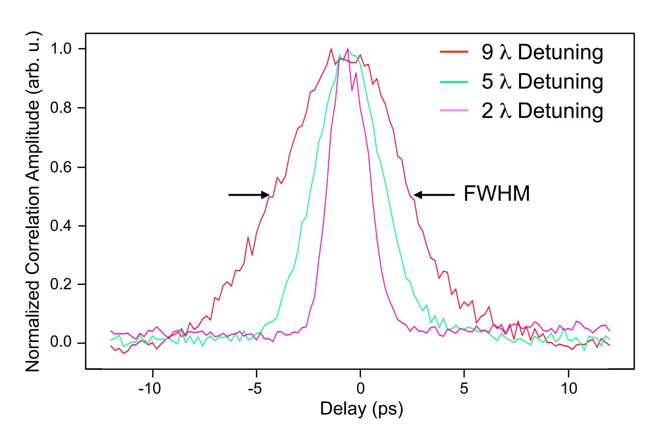
FWHM of cross-correlation signals for 3 cavity length detunings (both MIR and FIR)
