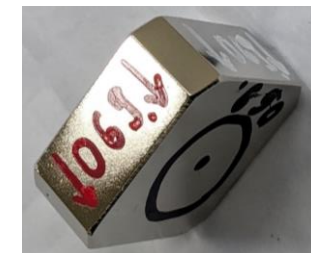
Magnet blocks. Size: 35 \times 35 \times 15 \text{ mm}^3
