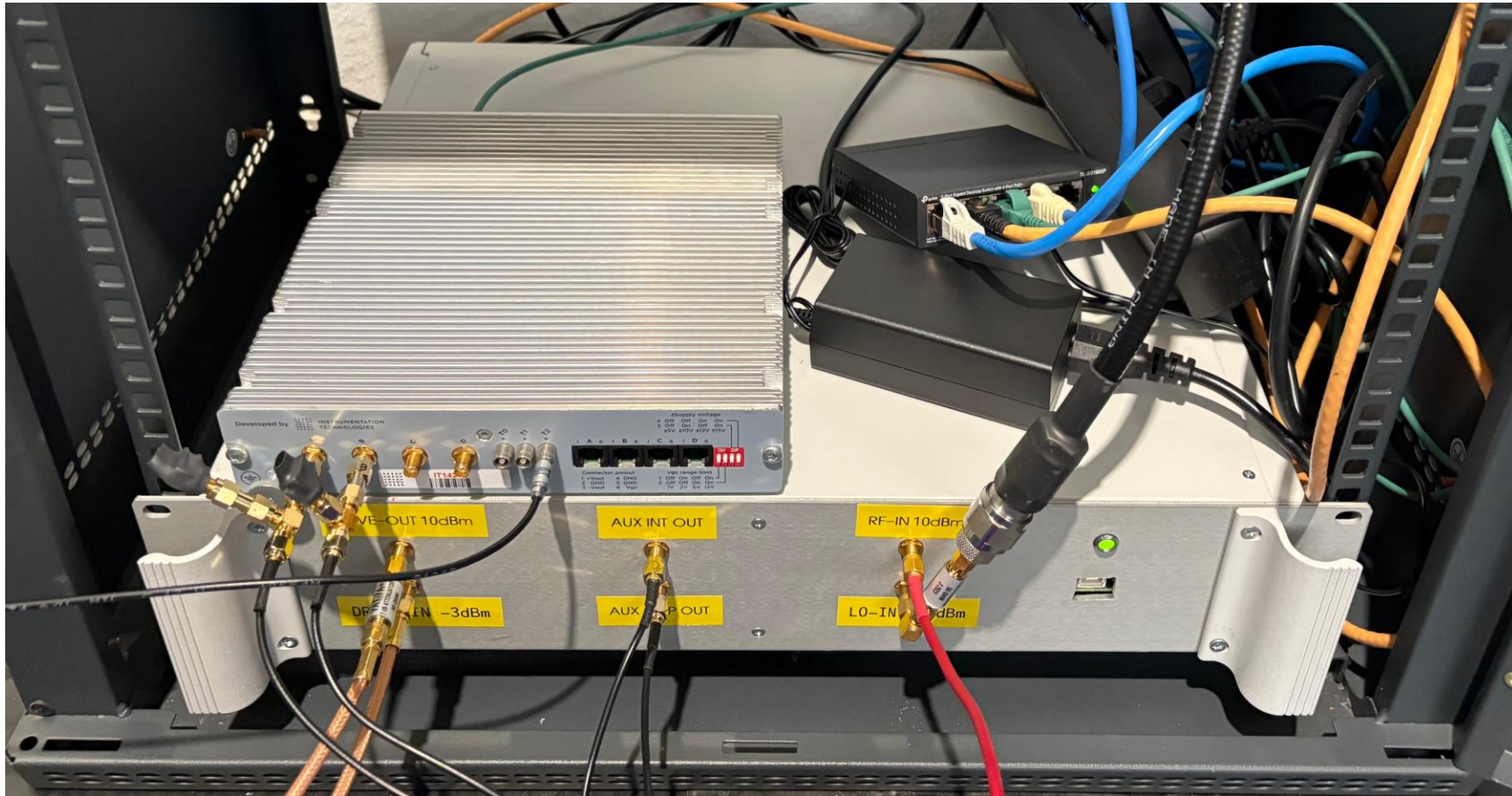
The Intra-Pulse feedback prototype and the Libera RF Digitizer used for the diagnostics.
